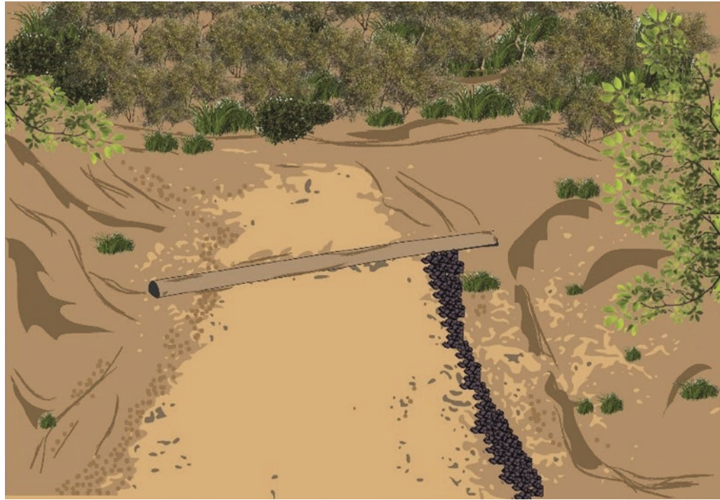
FIGURE 10.1 Water bar in place
